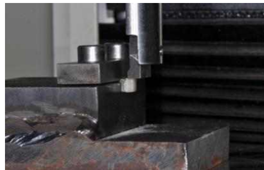
Fig. 3. Measuring of shear bond strength.
