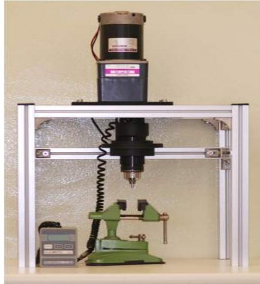
Fig. 7. Detorque value measuring set. This is composed of a digital torque gauge, an aluminum framework, a specimen loading apparatus, and an electronic grip.
