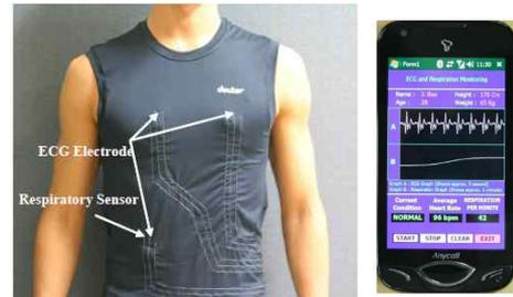
Figure 2. Smart clothing system for measurement of ECG and respiration(eong-Do Kim, et. al., 2010)
