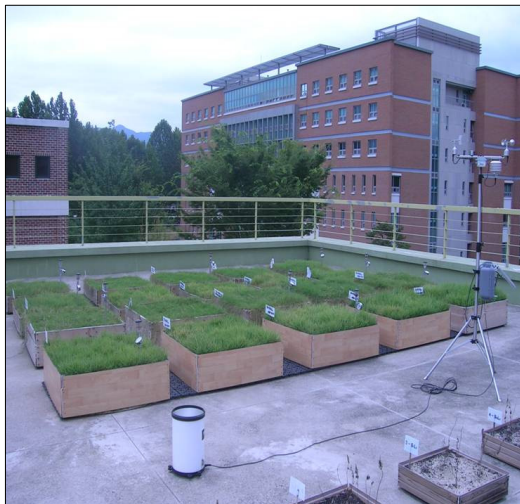
Fig. 1. The overall view of the experimental green roof with different growing substrates and soil depths on the rooftop.
