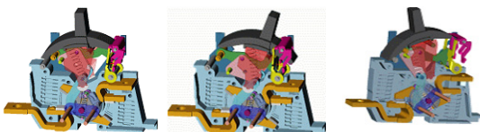
(a) Trip position (b) Open position (c) On Position Figure 2: Status of MCCB mechanism
