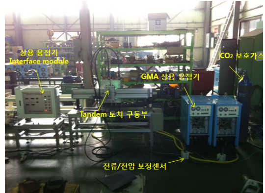
Figure 1: Tandem welding system using CO 2 shielding gas.
