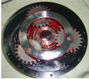
Fig. 3 Made-to-measure reduction-gear set
