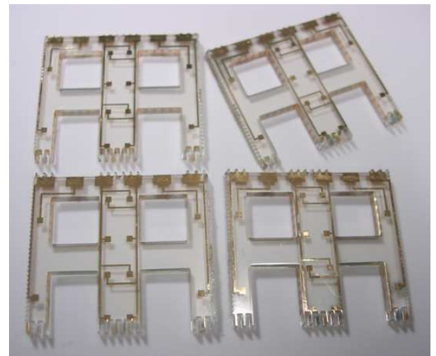
Fig. 3 Separated AEO3000 structure after gold sputtering for electrode fabrication
