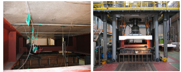
Fig. 4 Installation of gauges and actuator for testing
