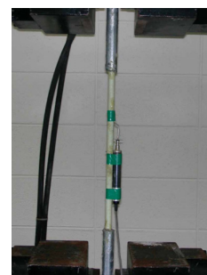
Fig. 6 Overall view of test set-up for tensile tests
