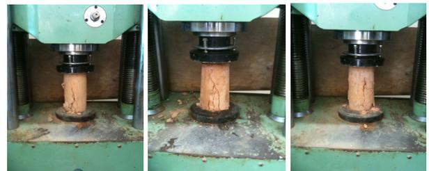
Fig. 4 Failure for Hardened Loess Specimen
