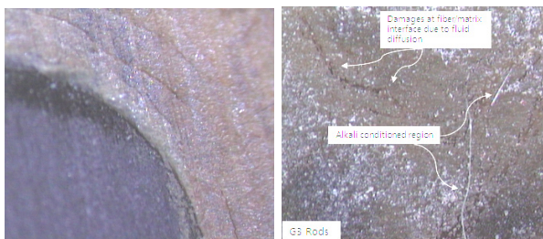
Fig. 9 Micro-images of immersed FRP rebars by alkaline solution
