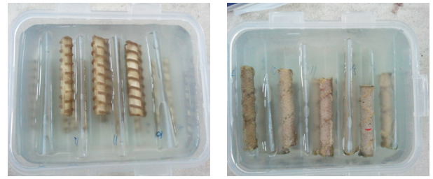
Fig. 5 Immersed FRP rebars in solution
