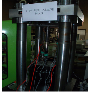
(b) Lattice girder ready for testing
