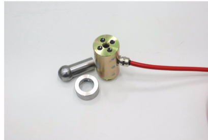
(b) Four strain gauges installed in the load cell
