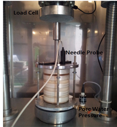
Fig. 2. Constant Rate of Strain (CRS) consolidation apparatus.
