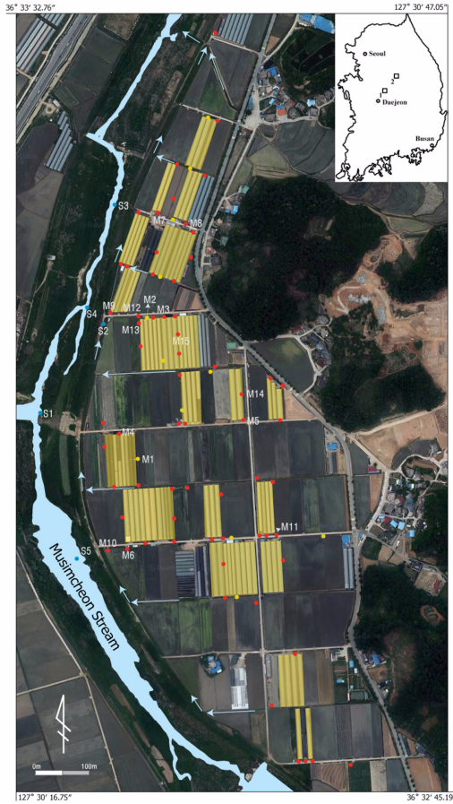
Fig. 1. Location of monitoring wells and discharging water flow in the Cheongweon water curtain cultivation area (No. 1 area on the index map). Red circles (M1-M14), wells equipped with a pumping system; yellow circles, wells without a pumping system; yellow rectangles, vinyl houses operating with water curtain cultivation; sky-blue arrows, flow direction of discharging water; blue circles (S1-S5), surface or discharging water.
