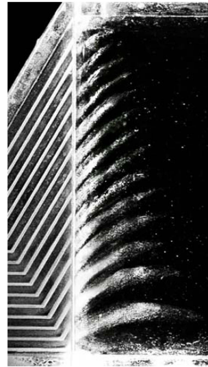
Fig. 9. Flow visualization of distributor outlet using hydrogen bubble method.
