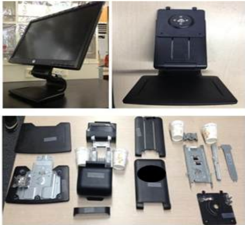
Fig. 4. Exploded components of benchmarking monitor stand.
