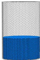
Fig. 8 25,100 contacted spheres in a cylinder model
