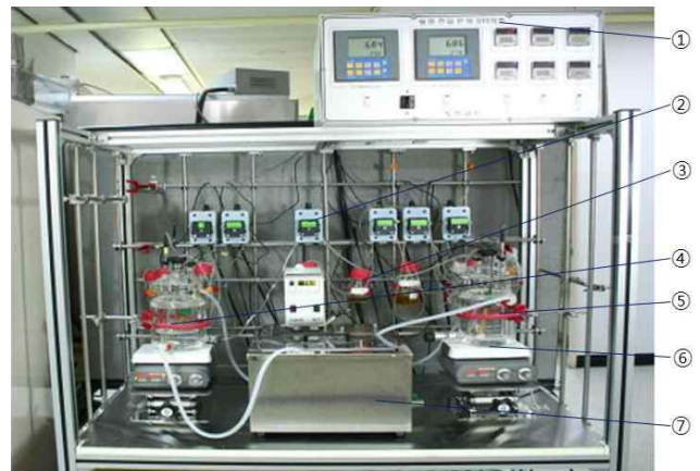
Fig. 1. Apparatus of stimulated human intestinal model system (SHIMS). (1) Control system (pH & pump); (2) Peristaltic pump; (3) Gastric & intestinal fluid, HCl, bile salt; (4) Stomach vessel; (5) Small intestine vessel; (6) Magnetic stirrer; (7) Temperature controller.
