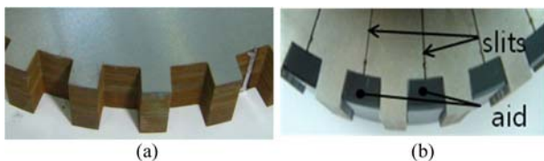
Fig. 2. (Color online) Fabricated stator outer core. (a) Core without slits, (b) Core with slits.
