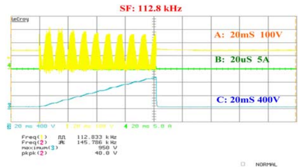
Fig. 9. (Color online) Charged waveform during 112.8 kHz switching frequency, and the measurement waveform overlapped during 20 mS 100 V of A, 20 \mu S A of BA, and 20 mS 400 V of C.
