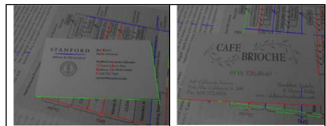
Fig. 21. Some failure results of card position localization of business cards.
