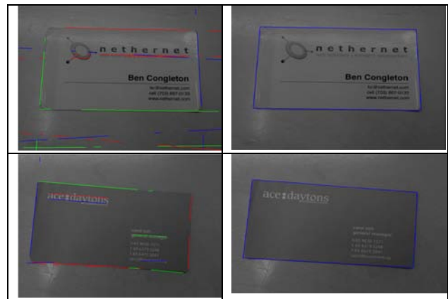
Fig. 5. Line detection results and shape position localization results.
