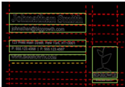
Fig. 12. Local region localization based on projection histogram.
