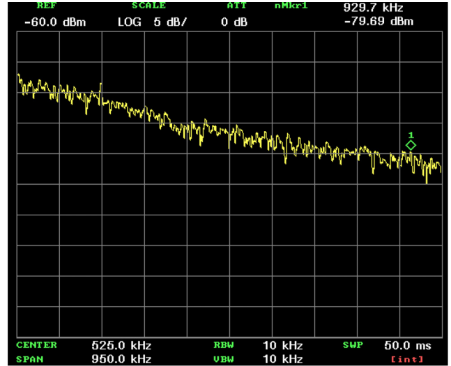
FIG. 7. The frequency response of the sensor.
