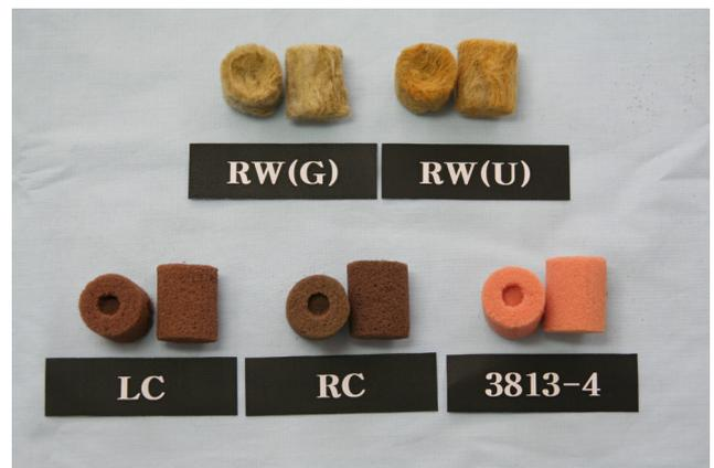
Fig. 1. Five pellet type media used in the experiment. RW (G), grodan rockwool (Grodan Co. Ltd., Denmark); RW (U), UR rockwool (UR Co. Ltd., Korea); LC, phenolic foam LC (Smithers Oasis Korea Co. Ltd., Korea); RC, phenolic foam RC; 3813-4, phenolic foam 3813-4.
