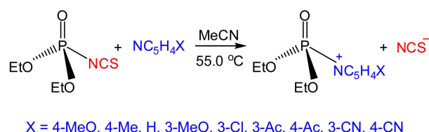
Scheme 1. The pyridinolysis of diethyl isothiocyanophosphate (1) in MeCN at 55.0 °C.
