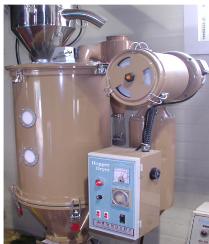
[Fig. 2] Hopper used raw material to drying and preliminary heat.
