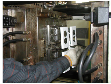
[Fig. 5] The injected acrylic plate from a cast.
