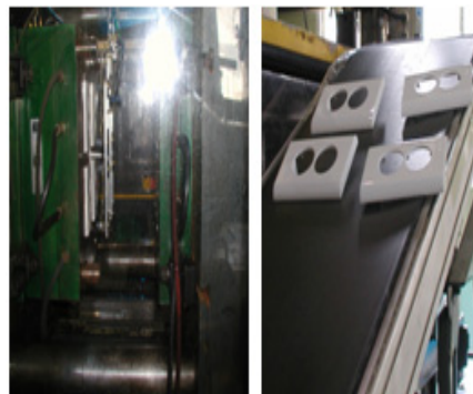
[Fig. 14] Using robot injected the acrylic plate from a cast.
