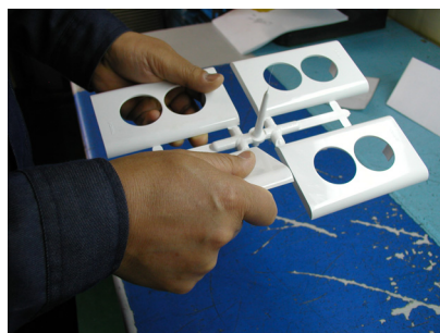
[Fig. 7] The separate sprue runner from the acrylic plate.
