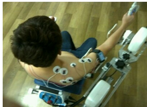
[Figure 1] The illustration of the EMG electrode placement.
