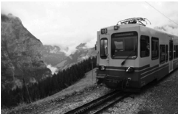
Fig. 3 Mountain train in Jungfrau driven by rack & pinion
