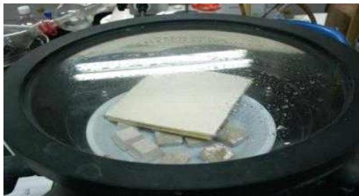
Fig. 3. Process route of square layer form of Ag-oyster bead[C-b] by vacuum dryer.
