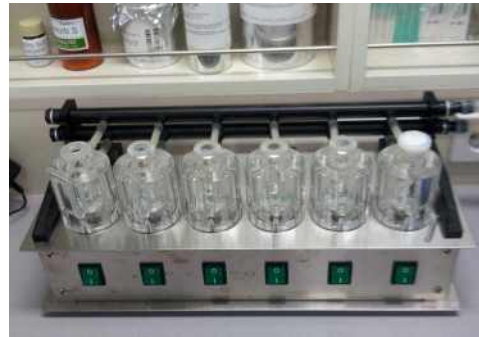
Fig. 1. Photograph of In Vitro transdermal absorption apparatus of drug release.
