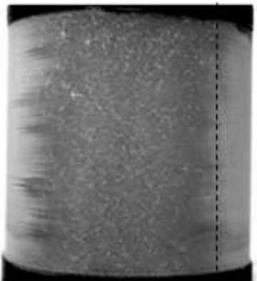
Fig. 7 Plating pattern appeared on the two cylinders, top view, P_v/D=1.5 (Turbulent)
