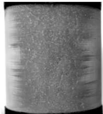
Fig. 7 Plating pattern appeared on the two cylinders, top view, P_v/D=1.5 (Turbulent)
