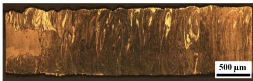
Fig. 10 Structure of longitudinal section of laser welded specimen
