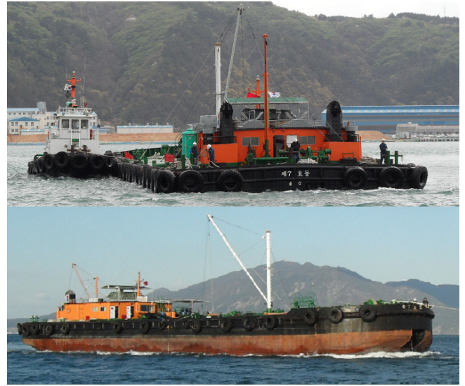
Fig. 6. Figure of barge(full load & ballast condition)
