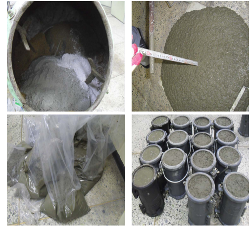
Fig. 2 Specimen preparation for compressive test
