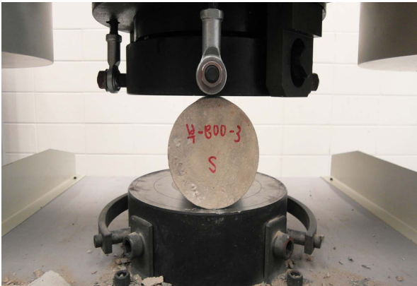
Fig. 5 Splitting tensile strength test
