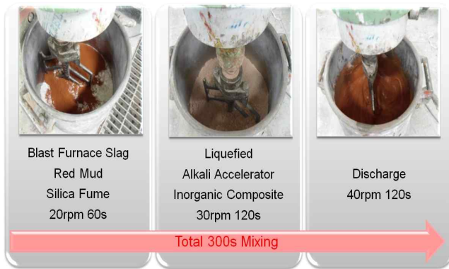
Figure 4. Mixing process of inorganic composite
