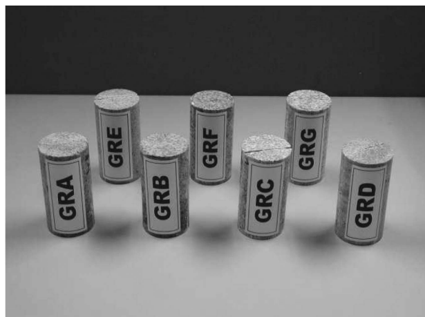
Fig. 1. Core Specimens used for the Measurements of Roughness
