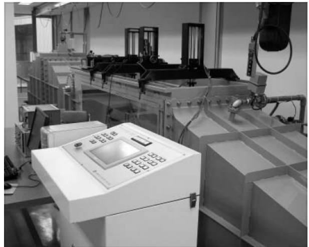
Fig. 5 Circulating water channel of the university of ulsan
