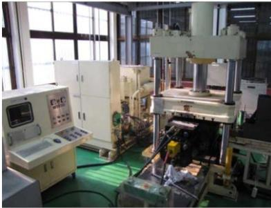
**Fig. 6 Hydroforming machine**
