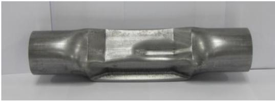
Fig.16 Hydroformed rectangular flange
