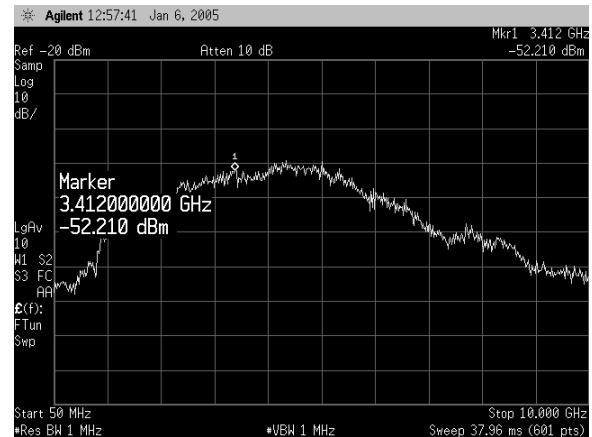
Fig. 2. Impulse UWB Signal Spectrum
