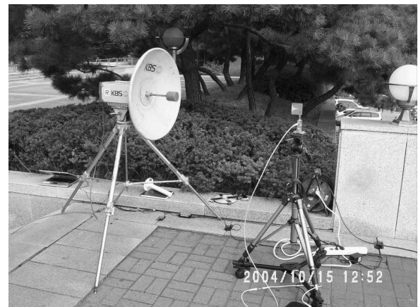
Fig. 7. Measurement set-up of interference between Broadcast relay and UWB
