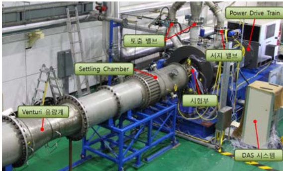
Fig. 5 KARI compressor test facility
