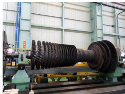
Fig. 3 Re-machining of damaged journal
