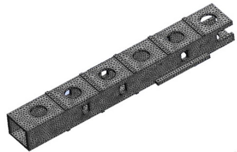
Fig. 3 Mesh structure of robot casting
