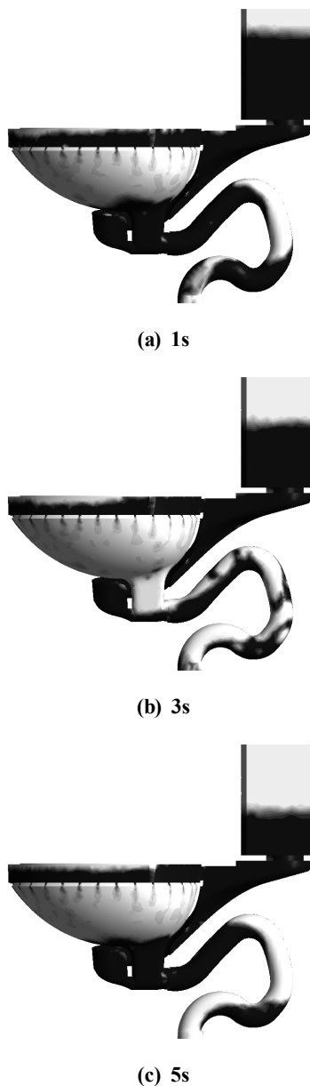
Fig. 11 Variation of water volume fraction with time for model 2 without remaining water
