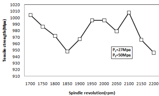
Fig. 8 Relationship between tensile strength vs. spindle revolutions
