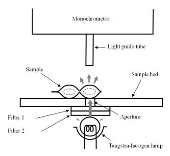
Figure 1. Optical layout of the developed NIR transmission spectrometer.
