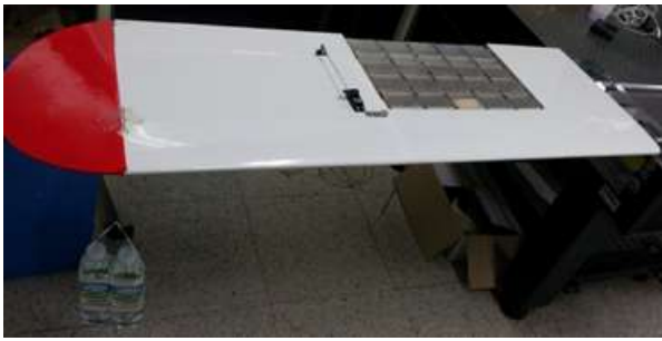
Fig.9 Load Test for deformation
