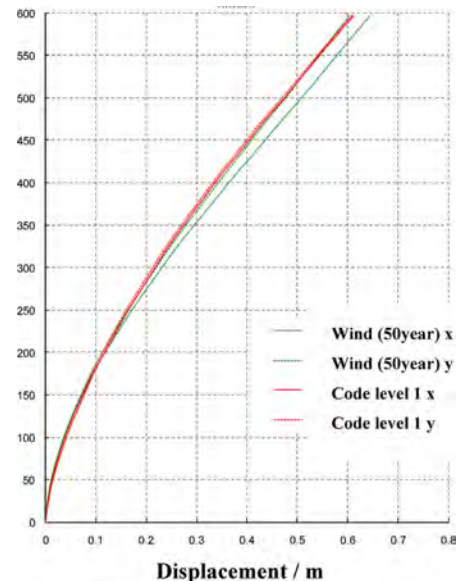
Figure 13. Displacement under earthquake and wind.
