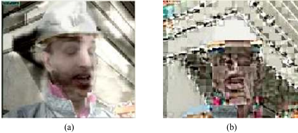
Fig. 8. Picture after encrypting DCT coefficients. (a) DC sign scrambling. (b) AC sign scrambling.
