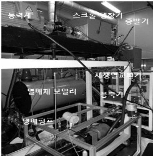
Fig. 10 Experimental set-up for ORC system.
